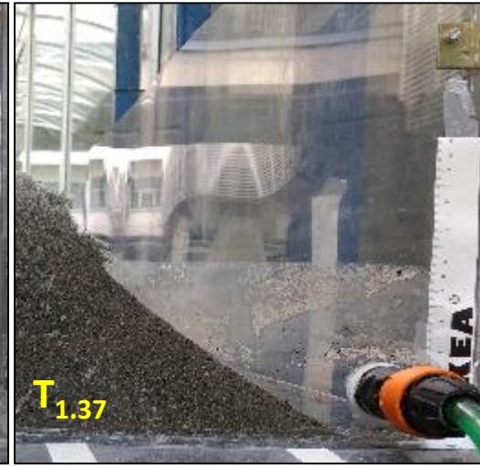
Sand material, simulating different water levels in the canal and various rainfalls
