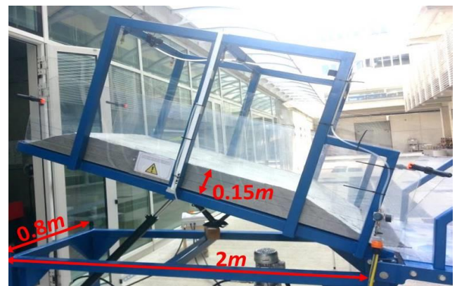
Fig. 1 – Geometry of the landslide simulator and sand layer.
