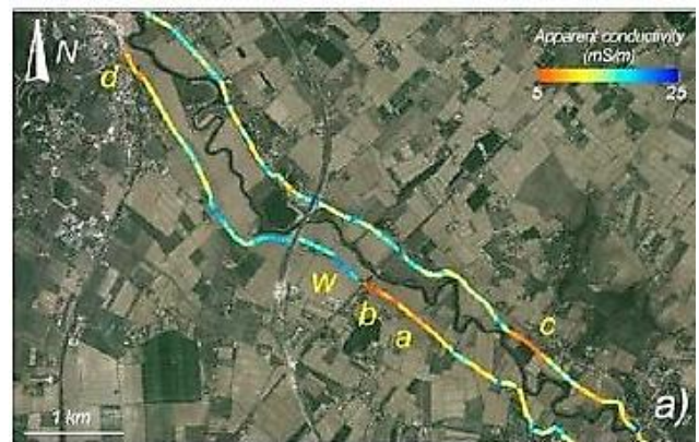
Figure 1: FDEM data showed four clear anomalies along Bacchiglione embankments (Francese and Monteiro Santos, 2014).
